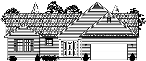
Elevation #2 Shown with Optional Window Grilles, K15 Style Front Door, Double Sidelites, 2 Car Garage and Porch
